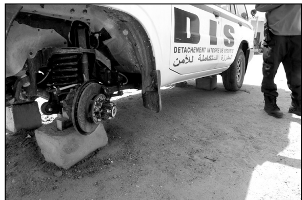
DIS vehicle with damaged suspension system. Bahai
